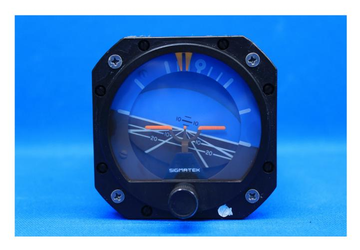
Air Craft Instrument showing the horizon with the nose and wing depicted set on the ground with a vacuum pump powered, gyroscopic with rigidity on 2 axis and some have a electric motor redundancy. You can now fly straight and level wings with the aircraft nose on the horizon. (whether you can see it or not as in IFR flights)
